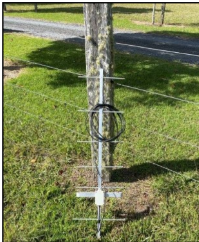
The overall winner was Larry Lindsay VK2CLL with his 7 element 70 centimetre yagi which achieved almost exactly the calculated gain.
