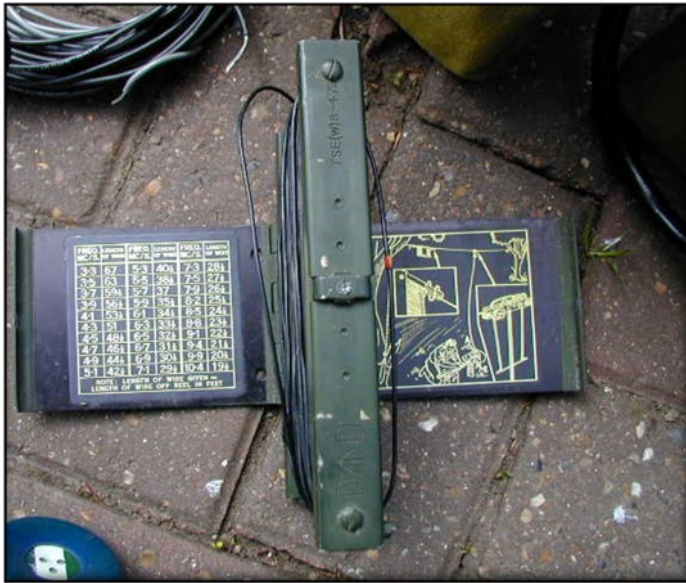
A510 DIPOLE ANTENNA ON METAL REEL. Note the red marker sleeve on the wire.
