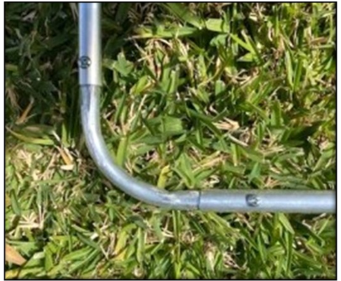
Securing the aluminium corners
