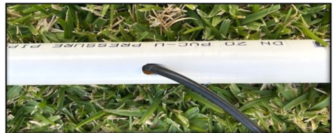
Feeding the coax into the boom
