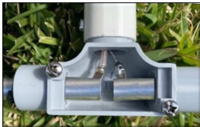
Ensure a 6mm gap between the driven elements
