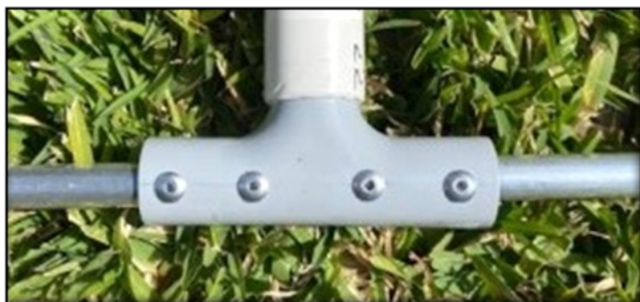
Securing the elements to the tee pieces
