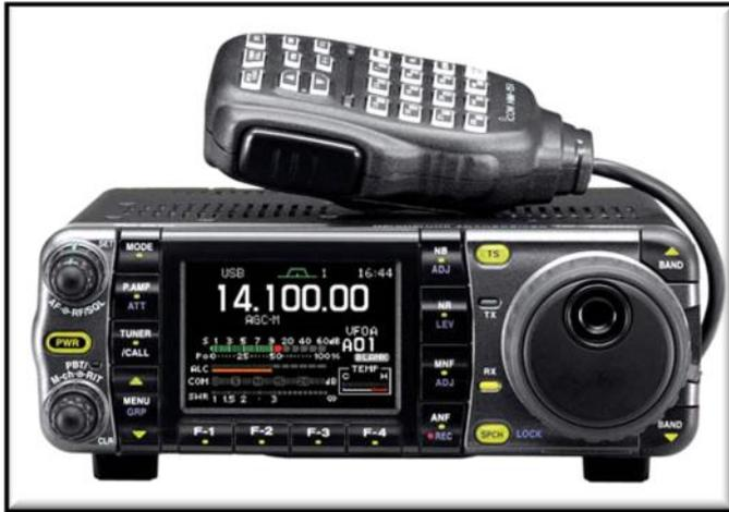
The **Icom IC-7000** was in production from 2005 to 2015. It represented the next generation in all-mode HF/VHF/UHF mobile transceivers. DSP at the IF level was the cornerstone of this multi-bander. The 7000 had two DSP chips to control bandwidths providing 41 bandwidths available as standard. Including being able to select sharp or soft filter shape.
