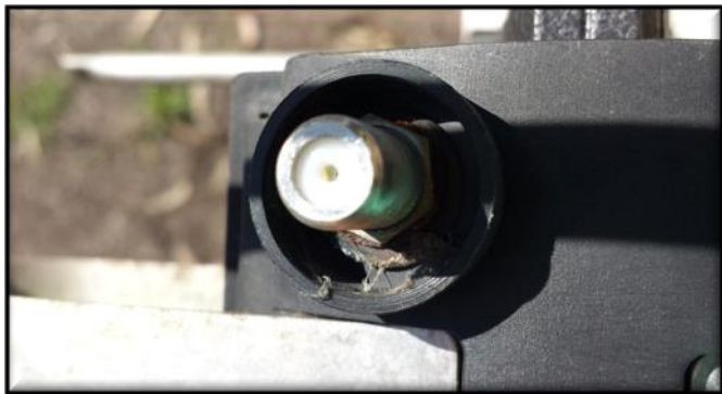
Photo 6 above: Corrosion around the UHF Yagi Balun “F” Connector
