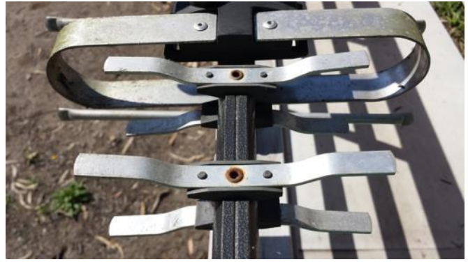
Photo 9 above: Aluminium Rivets in Driven Element, Steel Rivets in 1 st and 2 nd Directors
