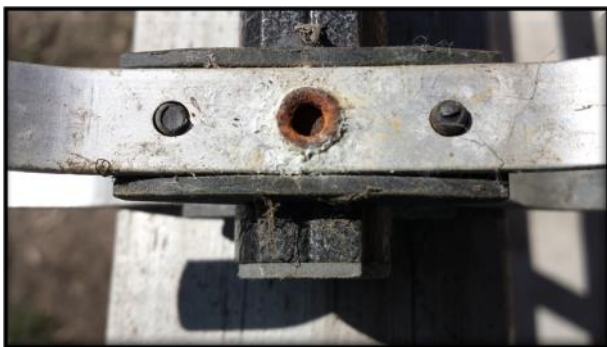
Photo 7 above: The Rust on the Rivets Fastening the First 3 Directors
