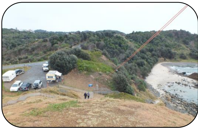
A 160 metre dipole is a long antenna. The same length of wire from the caravan extends up the distant hill.
