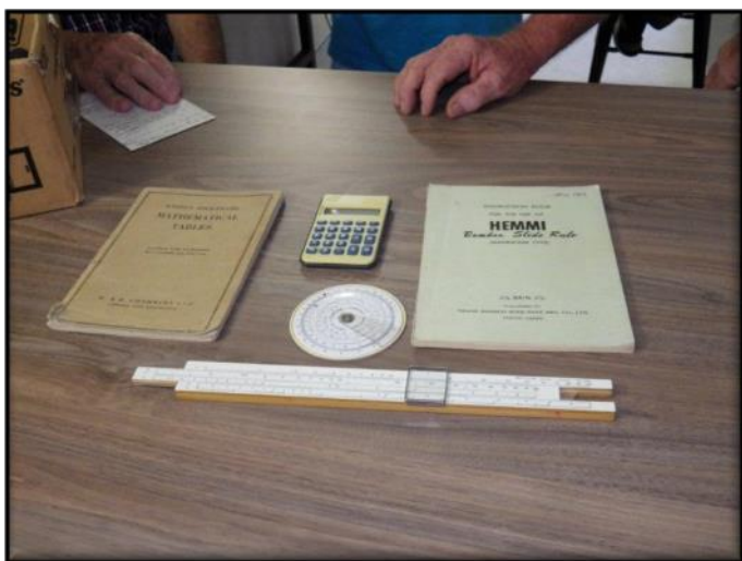
Mathematical Tables for logarithms (who can remember using those tables), Early basic electronic calculator, circular and linear slide room with a Hemmi instruction manual.
