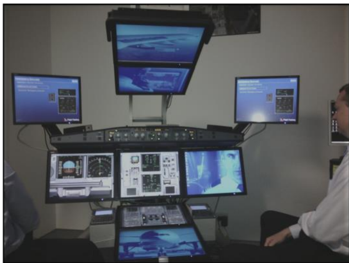
Figure 4: CAE Maintenance / Flight Training Device (MFTD) (During boot-up, all the screens are not yet active.)
