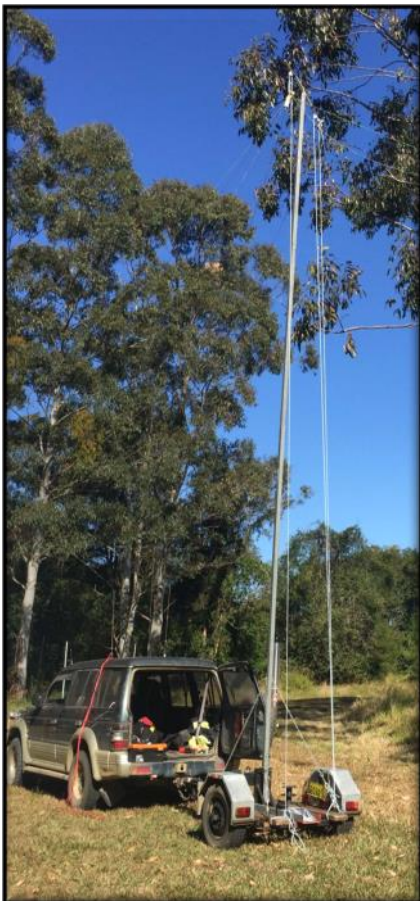
Lyle VK2SMI's trailer mounted mast and HF antenna. This antenna can be raised to a considerable height and also can be used as an anchor point for the various HF dipole antennas.
