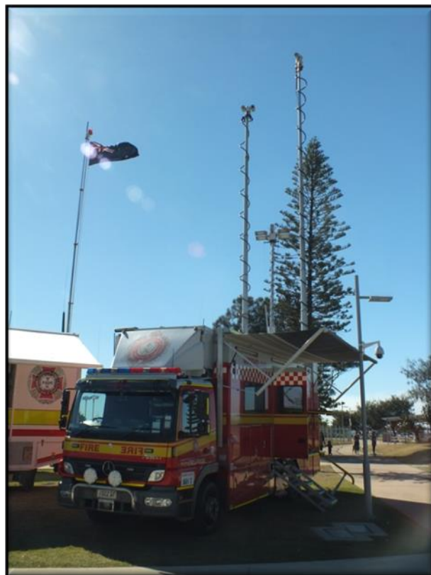
Above the Queensland RFS Command Unit and below the RFS Incident Control Trailer. Note LED lights on mast.
