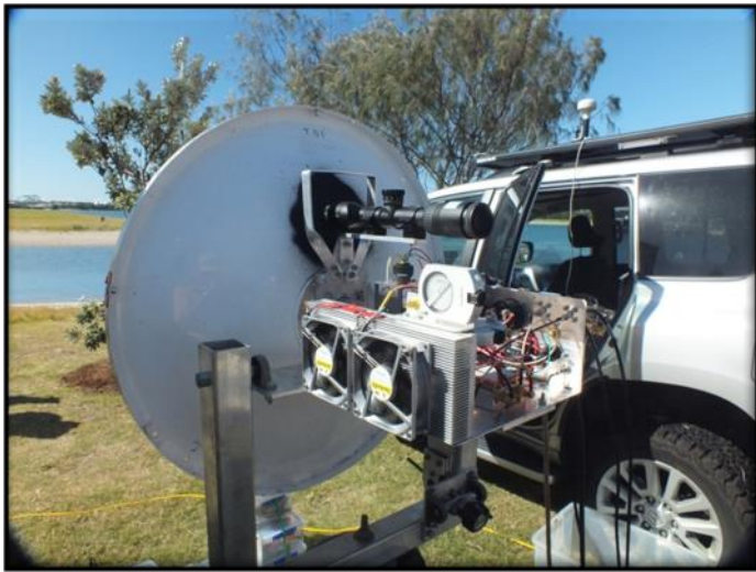
Rex VK7MO’s 10 Ghz RF Chassis. Note Rifle Scope sighting through the dish and GPS Antenna on 4WD roof.
