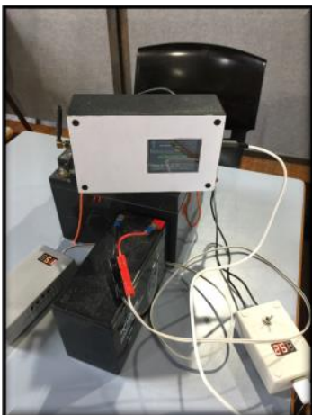
Portable Shark OpenSpot digital IP gateway operating through the mobile data network.
