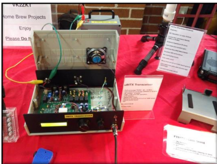
uBITX QRP HF all band SSB transceiver kit beautifully made up Gary VK2ZKT
