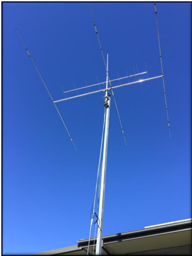
The 3 element HF beam to be moved. The object of the exercise was to gain greater clearance between the mast and the house. Stuart VK2FSU very kindly is donating the VHF beam to the club.
