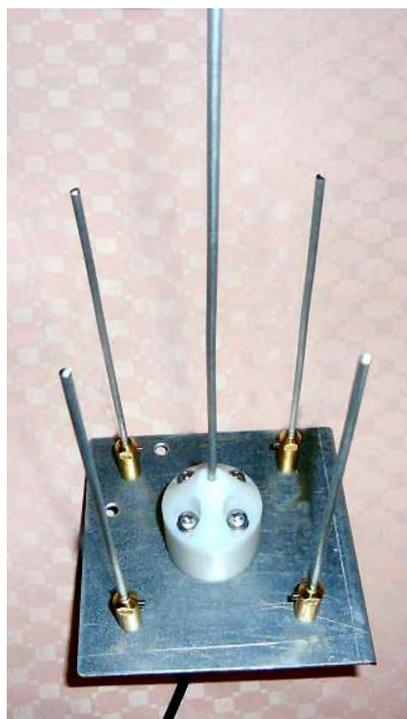
The antenna has a very broad band-width. Between the 2:1 VSWR points, it covered 390 to 430 MHz!
