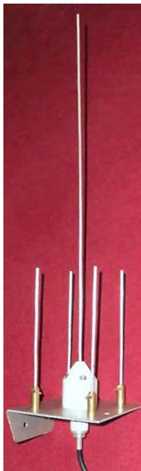
omnidirectional 2 metre antenna which needed no ground plane. It featured a main driven element, which was  $\frac{3}{4}$  wave length long, with 4 outer elements each of which were  $\frac{1}{4}$  wavelength long. The centre element was connected by coax to the transmitter. What fascinated me was the polar diagram of the radiation pattern; it was a near-perfect doughnut.
