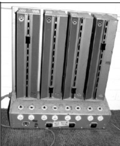
Old style resistive 8-channel dimmer unit
