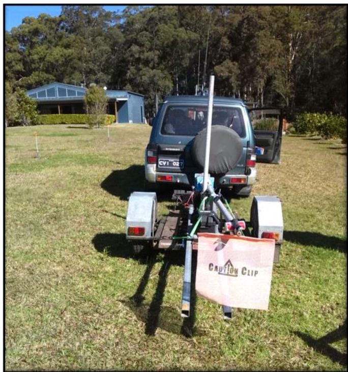
The very effective trailer mast built by Lyle VK2SMI in its transport position.
