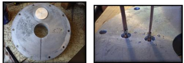
Blanking off redundant holes and drilling and tapping holes for coupling loop.
