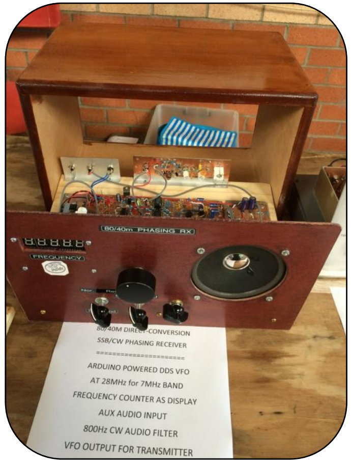
Home Brew 80 and 40 metre Direct Conversion SSB and CW phasing receiver.
