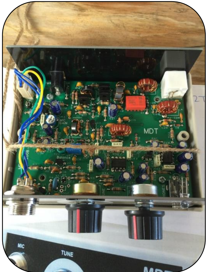
Home Brew 80 and 40 metre Direct Conversion SSB and CW phasing receiver.
