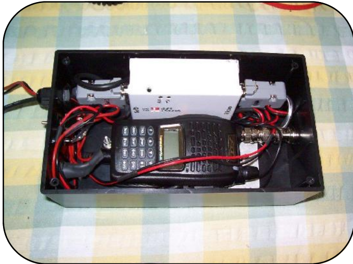
Internal view showing 2m transmitter, and interface unit with GPS receiver.
