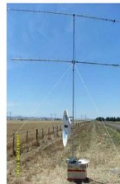
The portable antenna setup, 70cm, 2 mtrs & the dish.
