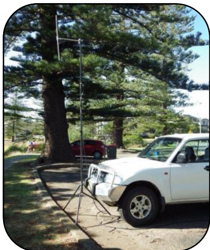
Portable repeater antenna on tripod
