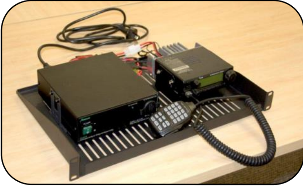
Echo Link Node equipment front view.
