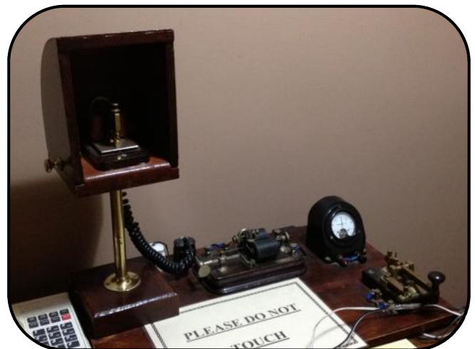
The Morse Sounder, sidewinder mechanical bug and straight key used to send Telegraphic messages (From the Beechworth Telegraph Office display).
